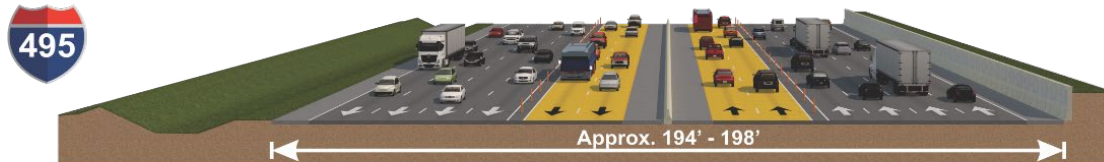
Figure 3-2: Alternative 9 - Phase 1 South Typical Sections (HOT Managed Lanes Shown in Yellow)
