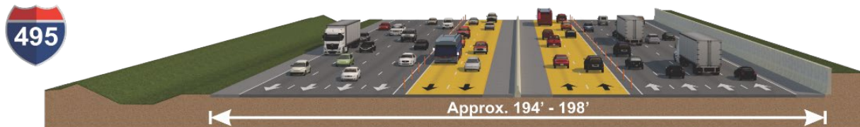
Figure ES-2: Alternative 9 – Phase 1 South Typical Sections (HOT Managed Lanes Shown in Yellow)
