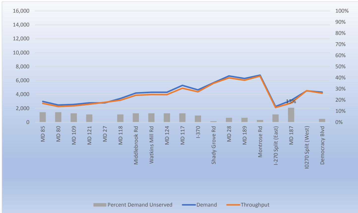
**Figure 5: I-495 2040 Diversion Alternative 4-5 PM Inner Loop Demand vs. Throughput and Percent Demand Unserved**
