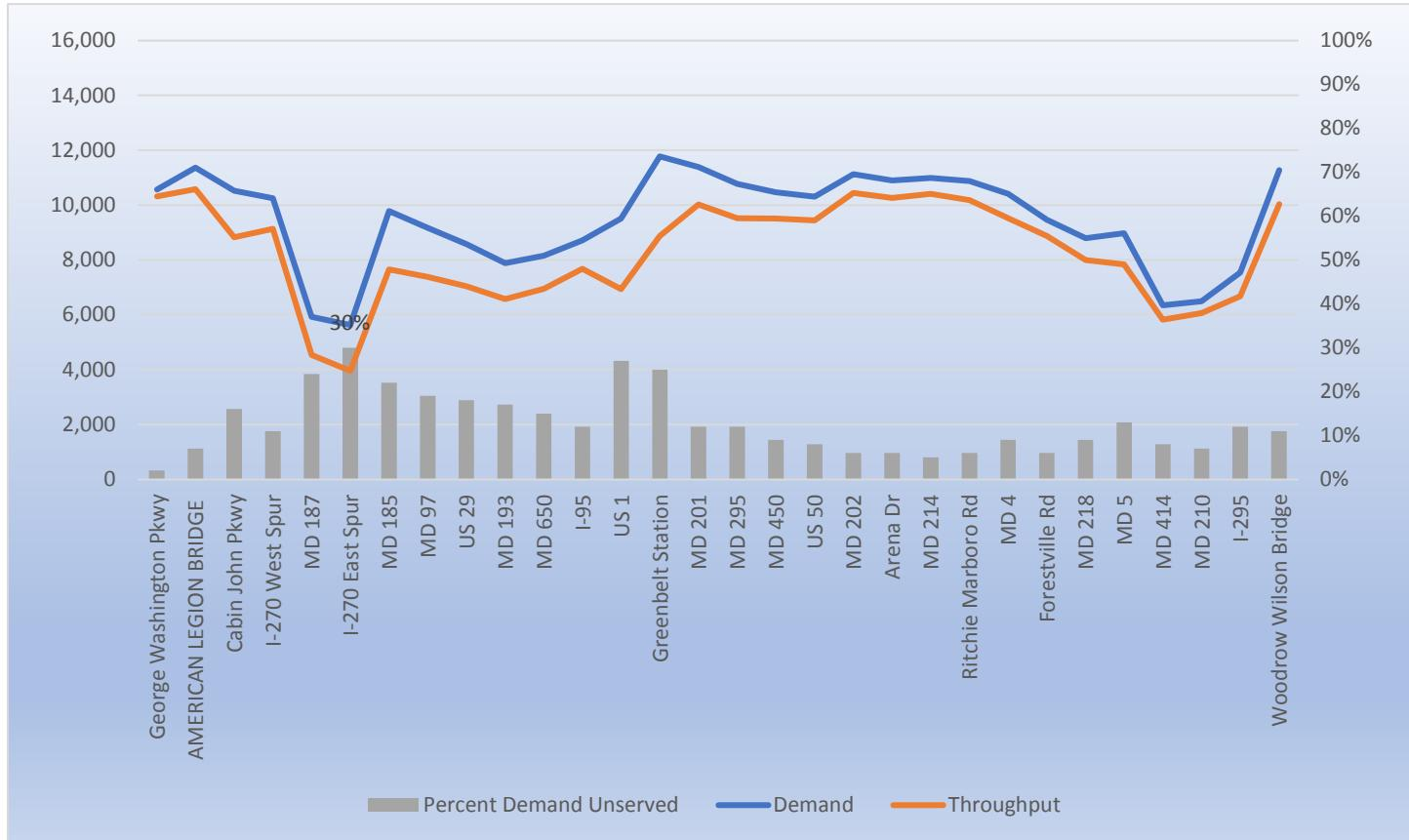
**Figure 2: I-495 2040 Diversion Alternative 7-8 AM Outer Loop Demand vs. Throughput and Percent Demand Unserved**
