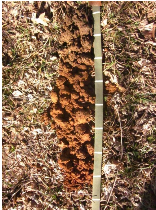
Figure 2. Although strongly developed, the thinness of the Boring 1 subsoil argillic horizon between the depths of 0.7 and 1.8 ft (20 to 53 cm) is suggestive of substantial grading.
