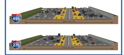
**ALT 13C:** 2 ETL Managed Lanes on I-495 and Reversible ETL Managed Lane plus 1 HOV Managed lane on I-270
